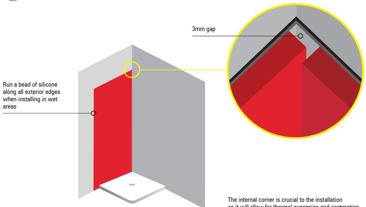
The internal corner is crucial to the installation as it will allow for thermal expansion and contraction.
